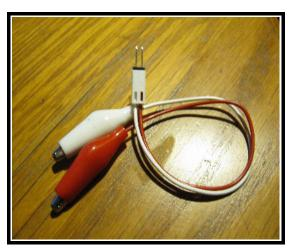
Turn a pair of alligator test leads into a test probe.
