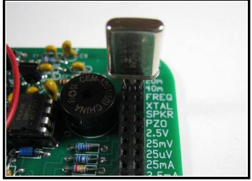
Testing a crystal in the FREQ slot.
