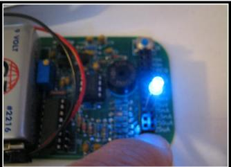
Use the 25uA, 250uA, 2.5mA & 25mA positions to test LEDs A regular LED will illuminate only faintly in the 25uA position, dull in the 250uA position and won't develop any real brightness until at least the 2.5mA test. A SUPER bright LED, like the blue one shown in the above pictures has noticeable lumens at the lowest 25uA position and will actually shock your eye when tested at the 25mA position.
